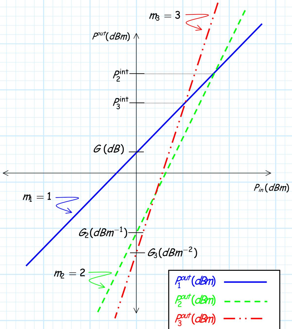
Note that for  $P_{in}$  (dBm)  $<$  0 dBm (the left side of the plot), the second and third-order products are small compared to the fundamental (first-order) signal.
